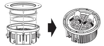
**NOTE:** The bolts that secure the frame to the body must be fully tightened in a uniform manner, alternating between diametrically opposed bolts. To facilitate the extraction of the glass without damaging the seal fitted onto the frame, unscrew all the nuts except for two adjacent ones and wait a few seconds; then unscrew the remaining nuts and remove the glass.
