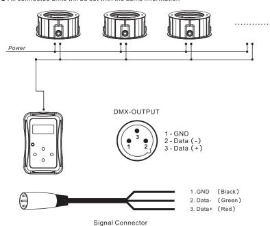
**Note:** The DMX Coder will automatically power off after extended periods of being idle (1 minute)
